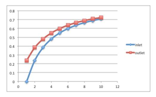
It is easily seen that you reach a point of diminishing returns – as the number of reactors increases each one makes a smaller contribution to the conversion.
